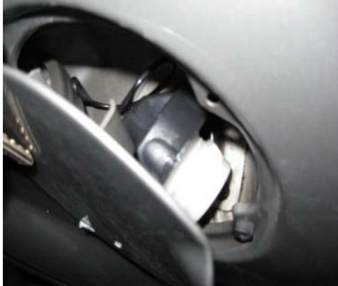
Gas cap off, 8 miles and 2 key cycles. The PCM still set an EVAP code even though the ambient air temperature was 20 degrees Fahrenheit, 20 degrees less than the criteria...
