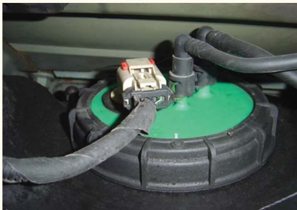
Chrysler Flex Fuel vehicles are easily identified by the presence of a green (vs. white) fuel pump module.
