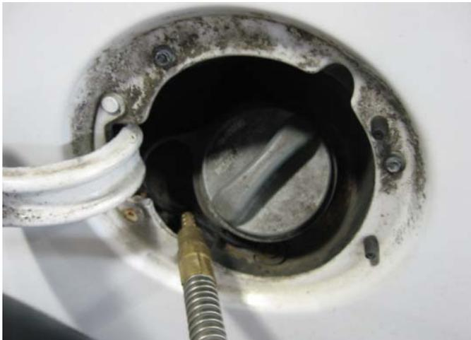
Waving the analyzer's probe around EVAP components that don't seal can result in evaporating hydrocarbons being drawn into the analyzer's probe.
