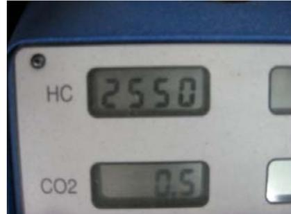
In this case the HC reading on the analyzer climbed to 2550 ppm when the probe was waved around the gas cap.
