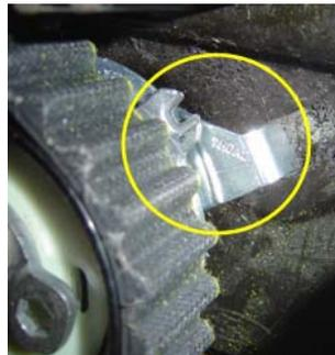
worth the extra effort. Correct tension allows the belt to stay centered on the pulleys and not destroy itself.
